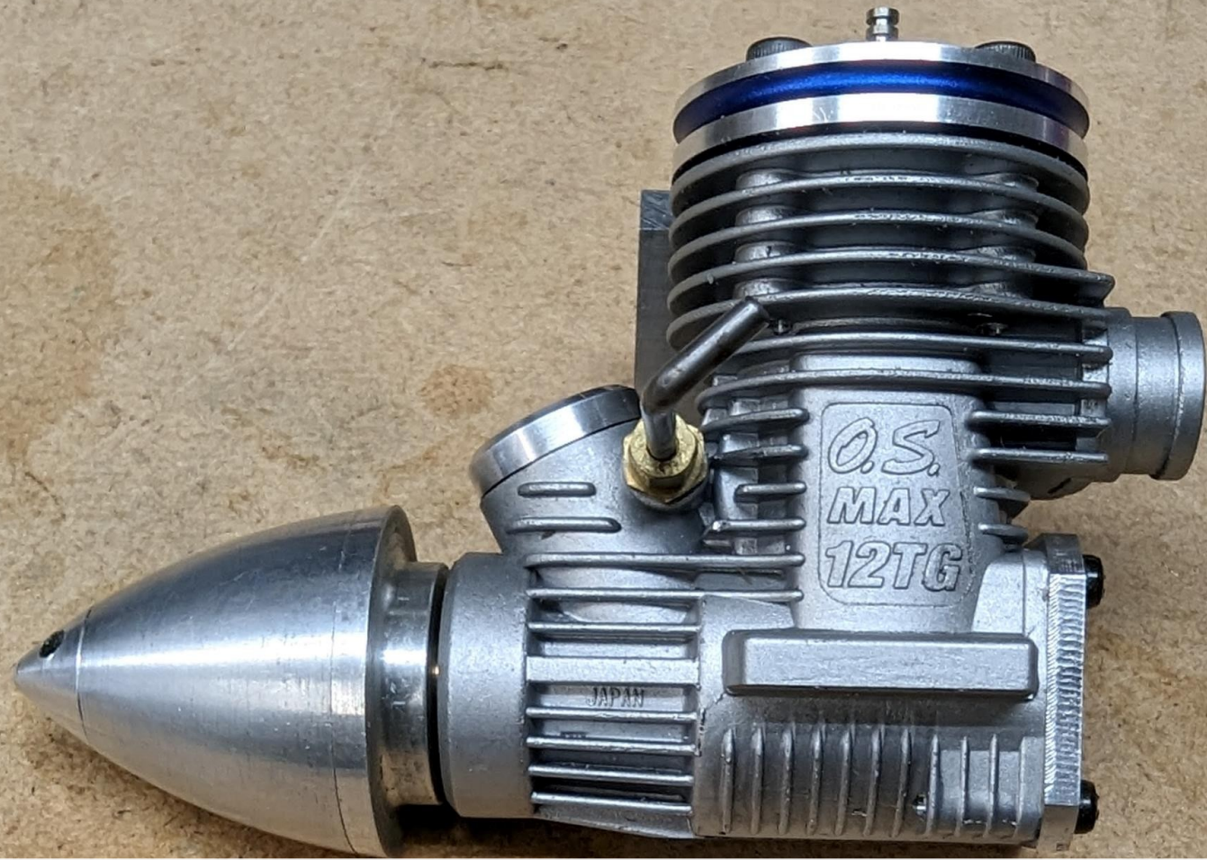
OS 12 MOTOR CONVERTED FROM A CAR ENGINE (Too short for a pan but ideal for a profile model)
